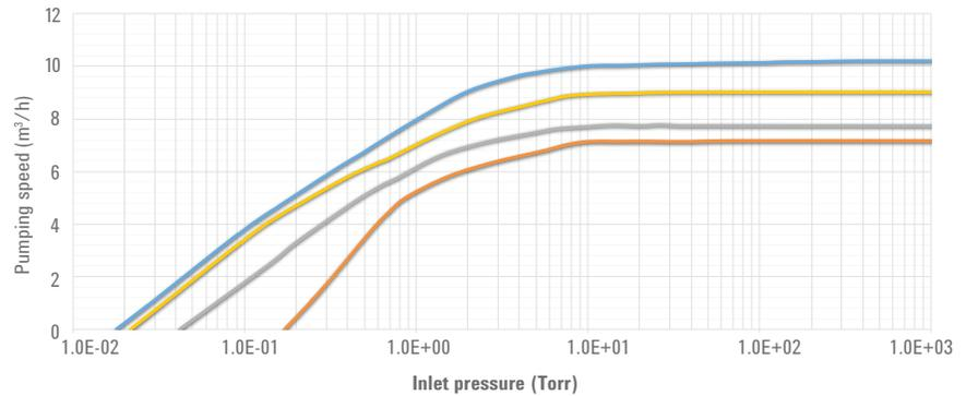
— 1900 rpm N<sub>2</sub> speed (m<sup>3</sup>/h) Factory set at 63.3 Hz
