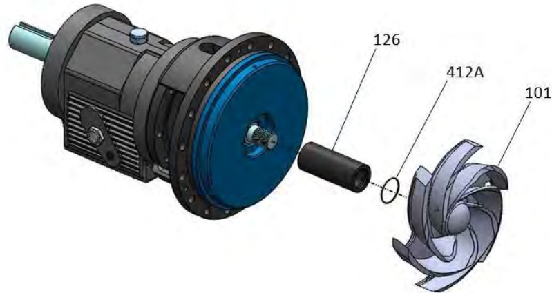
Figure 69: Shaft Sleeve installation
