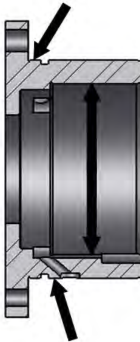
Figure 40: Inspection areas - Group 3 bearing housing
