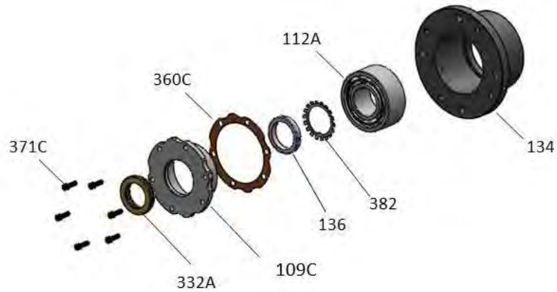
Figure 56: Bearing housing assembly – Group 4
