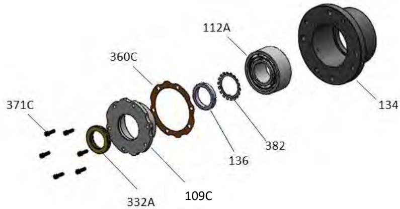
Figure 26: Bearing housing disassembly – Group 4
