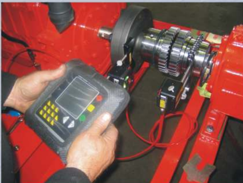
Laser alignment of couplings
