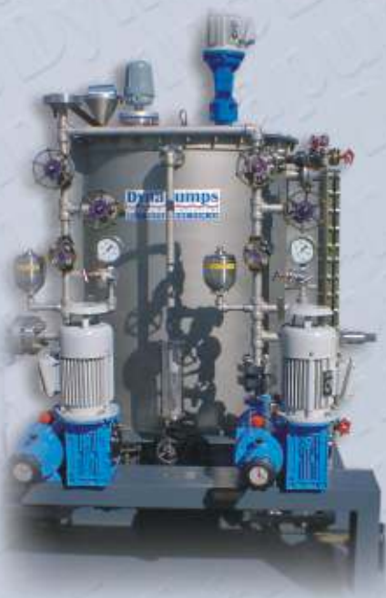
One of four injection skids for a fertiliser plant
