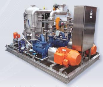
Duplex liquid ring pumps used to extract air from a steam condenser for the power generation industry – Queensland
