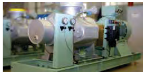
1 Crude Cargo Pump L4NG
