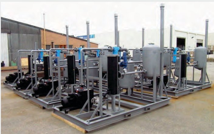
8 skids at the Dynapumps workshop ready for delivery
