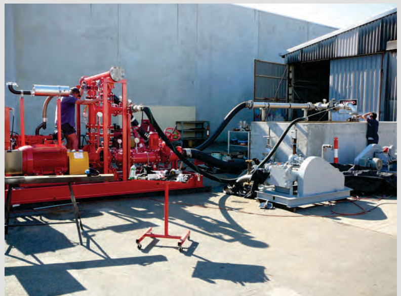
Above: Testing Pump on the Dynapumps testing system Above left: Preparing one of the packages for testing Far Left: Diesel Motor Left: Control panels to AS2941 standards
