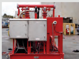
Above: Testing Pump on the Dynapumps testing system Above left: Preparing one of the packages for testing Far Left: Diesel Motor Left: Control panels to AS2941 standards
